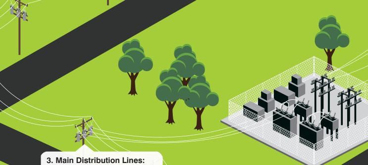
If the problem cannot be isolated at a distribution substation, distribution lines are checked. These lines carry power to large groups of consumers in communities or housing developments.
