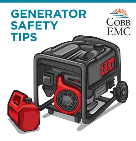
Never connect a standby generator into your home's electrical system. There are only two safe ways to connect a standby generator to your equipment.
